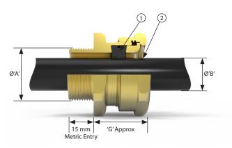
■1 Elastomeric Exd Flameproof and Exe Increased Safety seal on cable outer sheath
